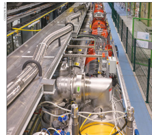
Cold-blooded The inner-triplet string under test at CERN's SM18 facility replicates, at full scale, the magnet chain that will focus the beams on either side of ATLAS and CMS. The flexible cryostat of the superconducting link, nicknamed "the python", runs alongside the platform, feeding the magnets with up to 120 kA through 19 MgB 2 cables.
