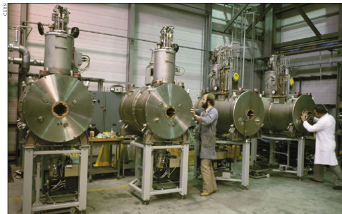
Cold quartet Four of the eight superconducting quadrupoles of the ISR's high-luminosity insertion, assembled in their liquid-helium cryostats at CERN.
