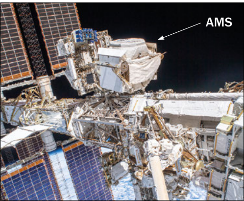
Above the clouds The view of ESA astronaut Luca Parmitano during a spacewalk to service AMS, in November 2019. The detector, wrapped in insulation, is attached to the ISS's main truss.
