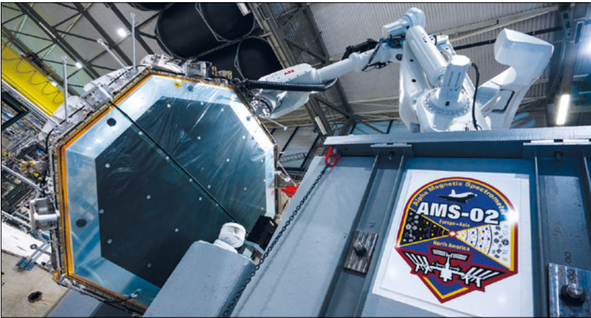
Fresh eyes The new silicon tracker layer for AMS, suspended from a robotic arm during proton-beam scans in CERN’s North Area. It is due to fly to the International Space Station in 2027.
