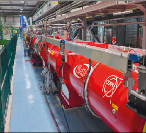
Niobium-tin The new quadrupole magnets for the HL-LHC reached nominal operating current at the IT String test facility.
