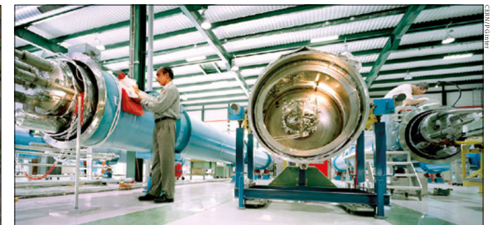
Mass production Cryostats for the LHC's main dipole magnets mid-assembly at CERN. The nearest is open, revealing the magnet wrapped in reflective insulation inside its blue outer vessel. More than 1200 were built, tested and installed in under a decade.
