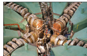
The 590 MeV ring cyclotron, the source of the proton beam that makes PSI's muons.
