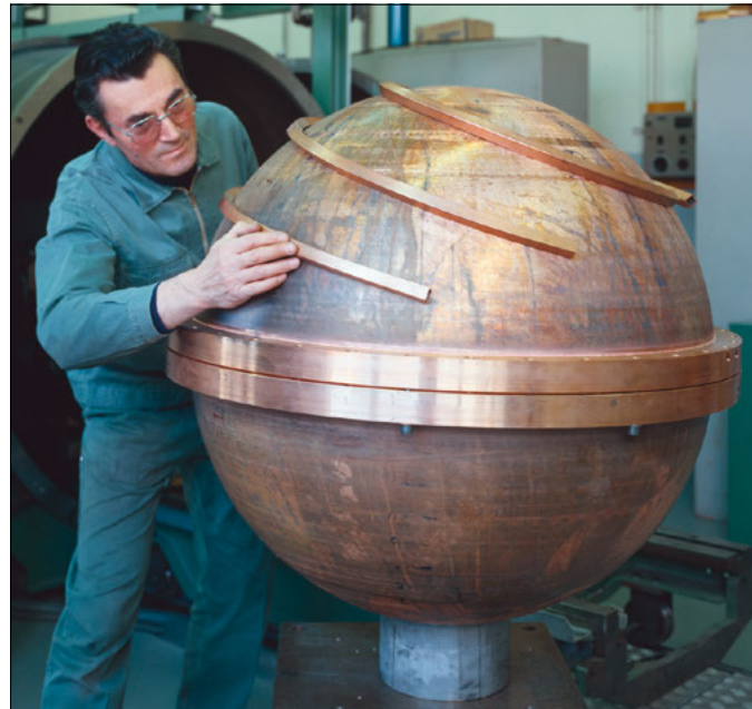
Balance of power A prototype storage cavity for LEP's copper radio-frequency system, photographed in 1980. The largest electron-positron collider ever built, LEP came of age at a time when particle physics had grown to a planetary scale.
