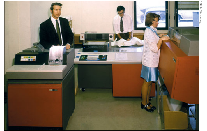
The first supercomputer The remote input/output station to CERN's CDC 6600 in 1972. The card reader on the left and the line printer on the right were operated by programmers on a self-service basis.
