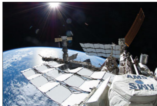
Safer space The Alpha Magnetic Spectrometer (AMS) on the International Space Station measures cosmic rays with high precision, generating data that also inform space radiobiology and radiation-risk for human spaceflight.
