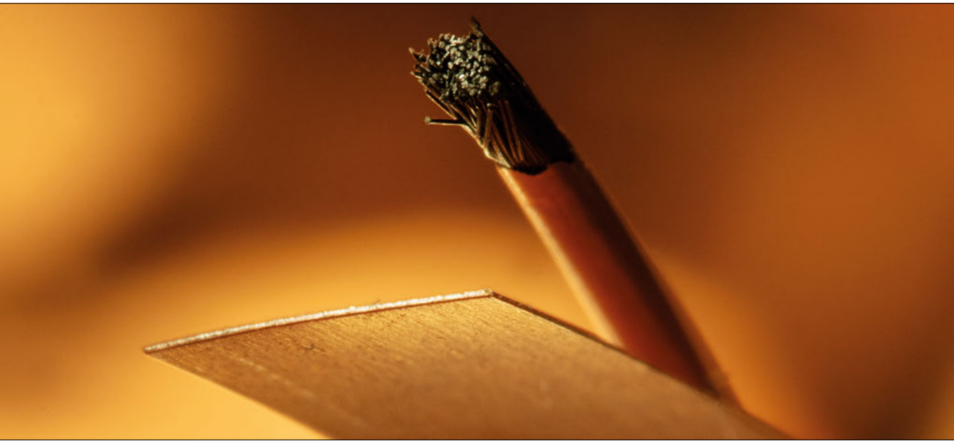
Frontier superconductors A closeup of a Nb 3 Sn wire and a 4 mm-wide REBCO tape. Both conductors can carry 500 A, but REBCO, a high-temperature superconductor, can withstand fields well in excess of 20 tesla at temperatures above 10 K. Credit: M Struik
