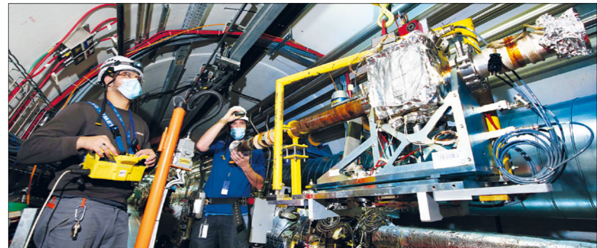
Heavy-ion collimation A crystal collimator is installed at the LHC, where it is used to deflect halo particles onto an absorber located roughly 90 metres downstream.
