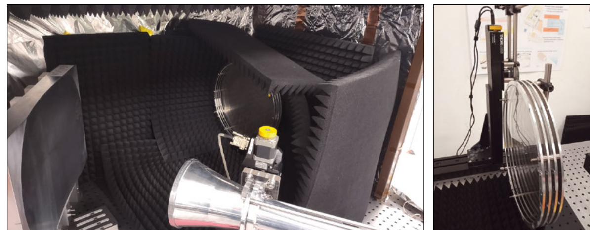
A work in progress A MADMAX prototype setup in the shielded laboratory at DESY/University of Hamburg. Microwaves from the booster (above, top right and enhanced image far right) are reflected from the focusing mirror (left) into a horn antenna (foreground right).
