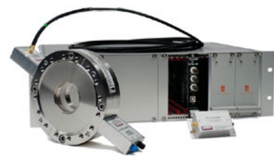
Fig. 2. The Integrated Current Transformer with dedicated analog electronics.
