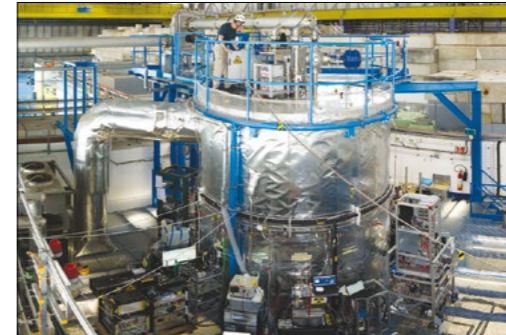
The CLOUD experiment CERN's Proton Synchrotron mimics the effect of cosmic rays on atmospheric gases.
