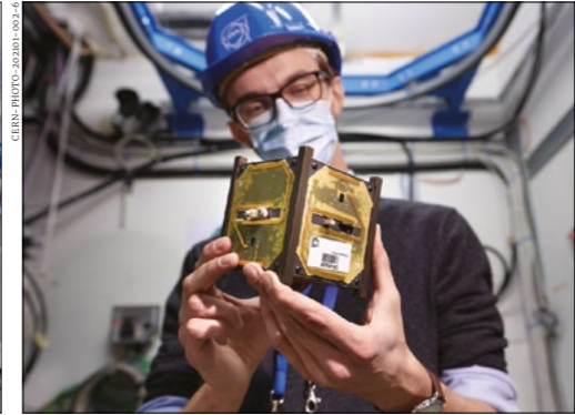
CubeSat A full-scale radiation-testing model of the CELESTA satellite.
