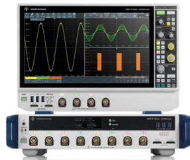
Fig. 1: MXO 5 and MXO 5C series oscilloscopes combined for more available channels.
