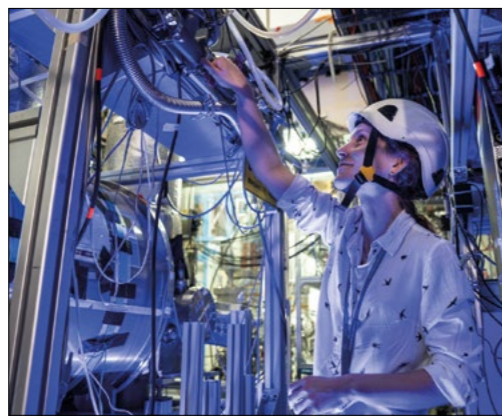
Flash frozen BASE physicist Barbara Latacz in front of the experiment's cryostat, which houses the system of traps used to cool and measure single antiprotons.
