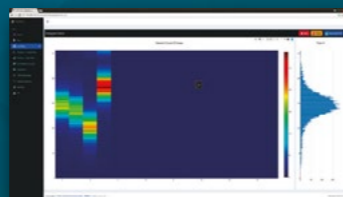
Position heatmap (counts over position) corresponding to four different 3 He tubes and 2D-projection of counts onto the y-axis of a single tube.
