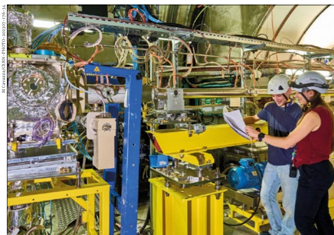
Rubidium source AWAKE's 10 m-long rubidium vapour source.
