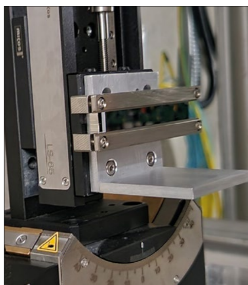
TWOCRIST crystal A 7 cm-long prototype precession crystal with a bending angle of 7 mrad.
