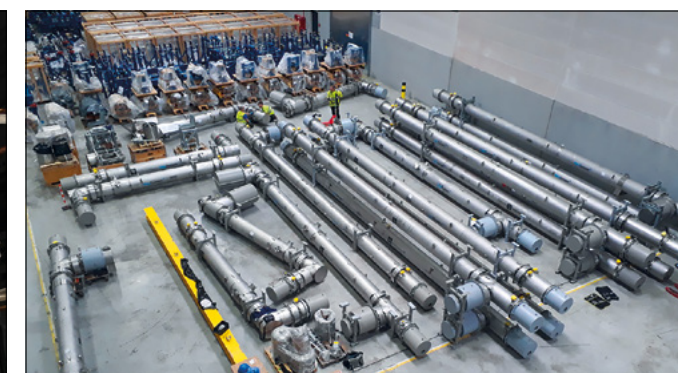
Cryo connections Above: Cryogenic by-pass lines supplied to FAIR through an in-kind contribution by WUST in Poland.
