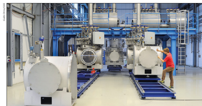
Test and measurement The STF (top) handled the volume testing of FAIR's SIS100 dipole magnets (110 in total). Meanwhile, CERN's specialist test facility (right) is overseeing acceptance of Super-FRS superconducting magnets prior to delivery to Darmstadt.
