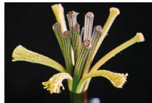
Flourishing A magnesium diboride cable, 19 of which are twisted together inside a compact, flexible cryostat to provide one of eight superconducting links powering the HL-LHC magnets.
