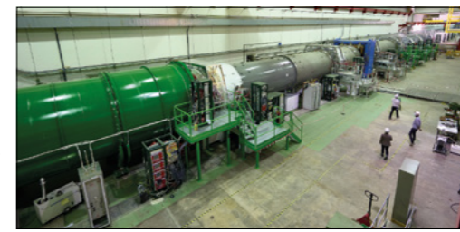
Intense Part of the NA62 detector in the ECN3 experimental hall in Preessin, where beam travels from right to left. On the right-hand side is the STRAW spectrometer, with the analysing magnet in blue. Four large-angle vetoes serving to clean the samples from non-forward events are visible in white, while the green region houses the RICH detector.
