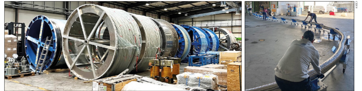
kA currents Delivery and handling of the 120 kA MgB 2 cable assembly. The flexible, double-walled corrugated cryostat comprises 19 MgB 2 superconducting cables in a single assembly, twisted together to form a compact bundle. Each MgB 2 cable is about 140 m long with the bundle diameter around 90 mm.
