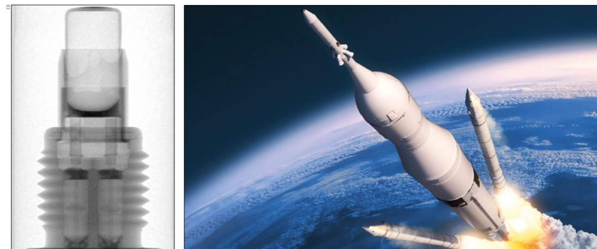
Feel the heat French aerospace company Dassault Aviation makes regular use of the ILL's neutron imaging capabilities, with the focus on radiographic analysis of high-reliability pyrotechnic equipment (left) destined for applications in rocket launchers (illustrated right).
