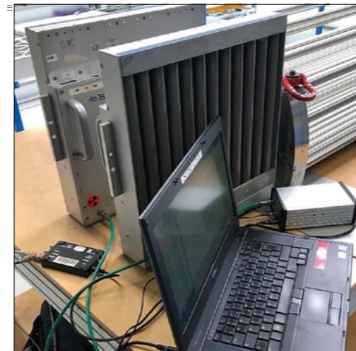
Flying high A custom ILL detector is currently being used by Airbus Avionics on commercial aircraft to measure the flow of thermal neutrons at different altitudes. The design, development and implementation of advanced neutron detectors is a core activity at ILL.
