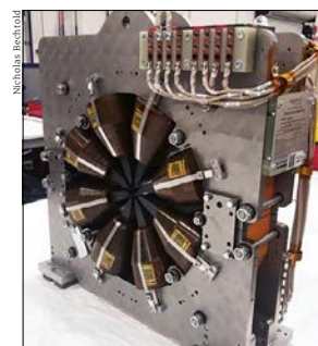
Beam steering An eight-pole fast-corrector magnet destined for the APS-U electron storage ring.
