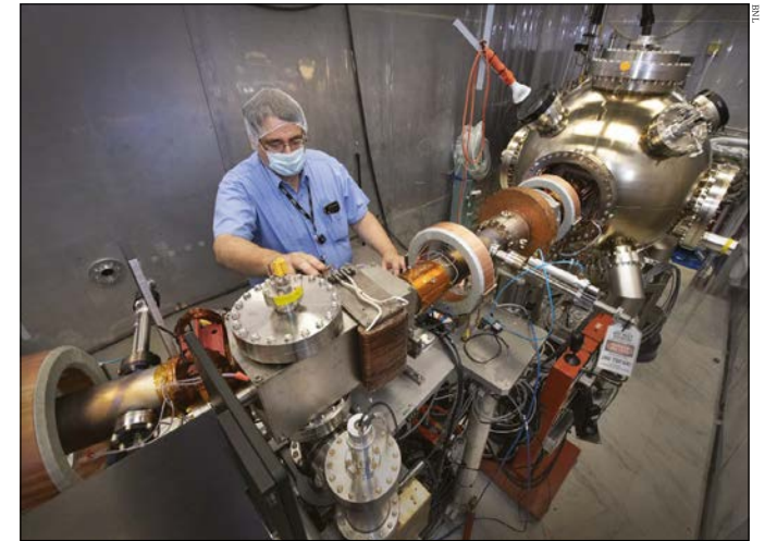
Test case The prototype bunched-beam polarised electron source, shown here in a recent test beam, achieved a peak current of 4 A with a bunch charge of 8 nC, meeting the EIC performance specifications.
