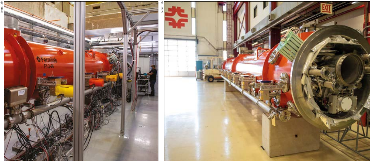
In the works Fermilab was the “designer of record” for the SRF cryomodule, with primary responsibility for delivering a working design to meet LCLS-II requirements. A cryomodule in the Fermilab test cave is put through its paces (left) before being prepared for transport (right) to SLAC.
