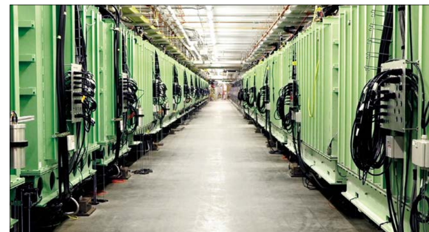
Going straight At the heart of the FRIB scientific programme is the 400 kW SRF linac. The heavy-ion accelerator comprises 46 cryomodules, assembled in-house by FRIB staff from industry-supplied components.
