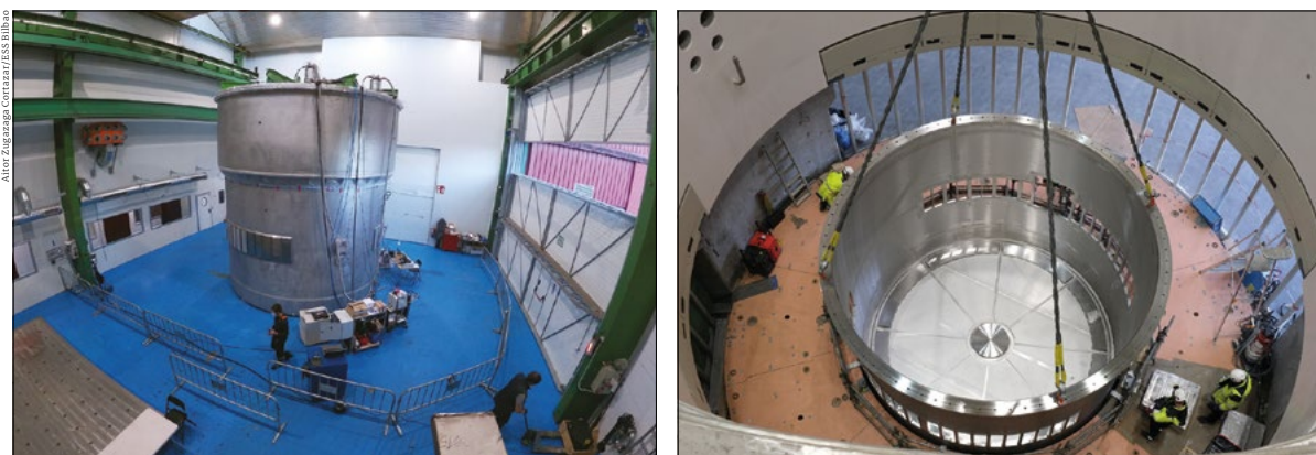
Heavy metal The TMV (left) represents the core building block of the ESS target station and was assembled by in-kind partners at ESS Bilbao, Spain, working in collaboration with local manufacturers. Ahead of shipping and installation into the target station (underway on the right), ESS Bilbao successfully completed the leak and vacuum tests on the TMV with satisfactory measurements of dew-point temperature, pressure rise and leak detection.
