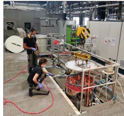
Bath time The Building 107 team has extensive experience in the electroplating of large vacuum components and can plate with copper, silver, nickel, gold and rhodium. The laboratory also provides custom surface-treatment services for other big-science facilities, including the electroplating of the above component for the Drift Tube Linac tanks of the European Spallation Source (ESS).
