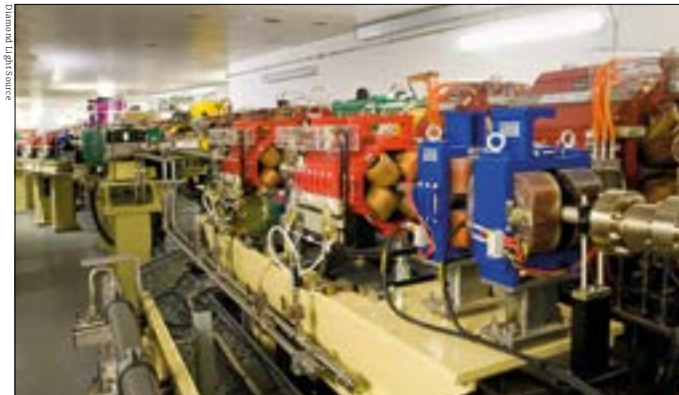
Intense X-rays The transfer lines at Diamond Light Source where ultra-relativistic electrons produce intense synchrotron radiation.
