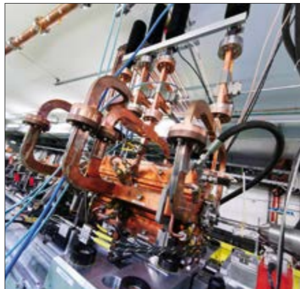
High-tech A dosimetry experiment for VHEE studies in collaboration with NPL (left) and a CLIC RF X-band cavity prototype (right) in CERN's CLEAR user facility.
